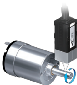
Eccentricity measurement of motors
